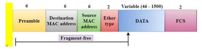
A Fragment-free switching is an advanced technique of the Cut-through Switching.
