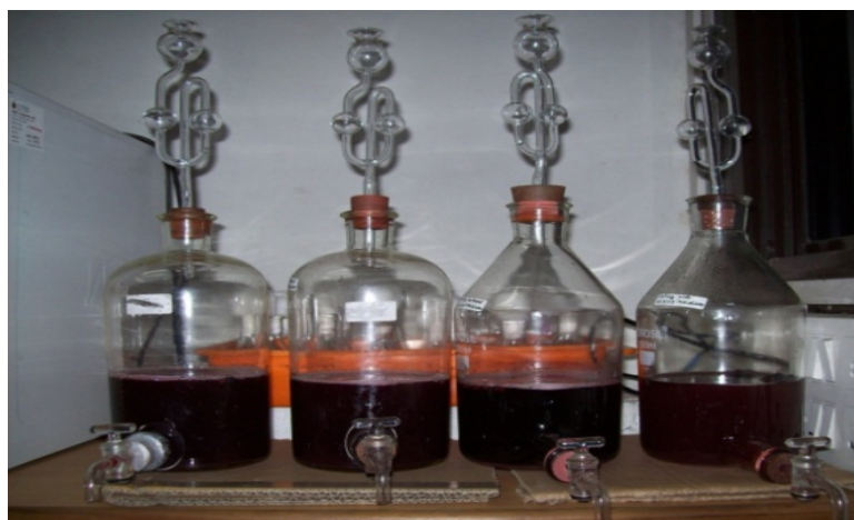
Fig. 3.7 Laboratory scale wine fermentation using Shiraz variety grapes
