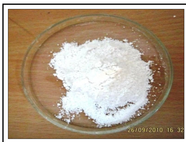
Fig.3.1 \text{CaSiO}_3 powder calcined at 1250^\circ\text{C}
