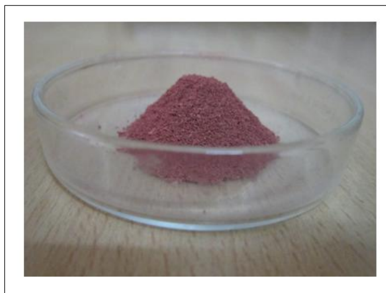
Fig.6.1 Fe-HAP powder calcined at 1000°C
